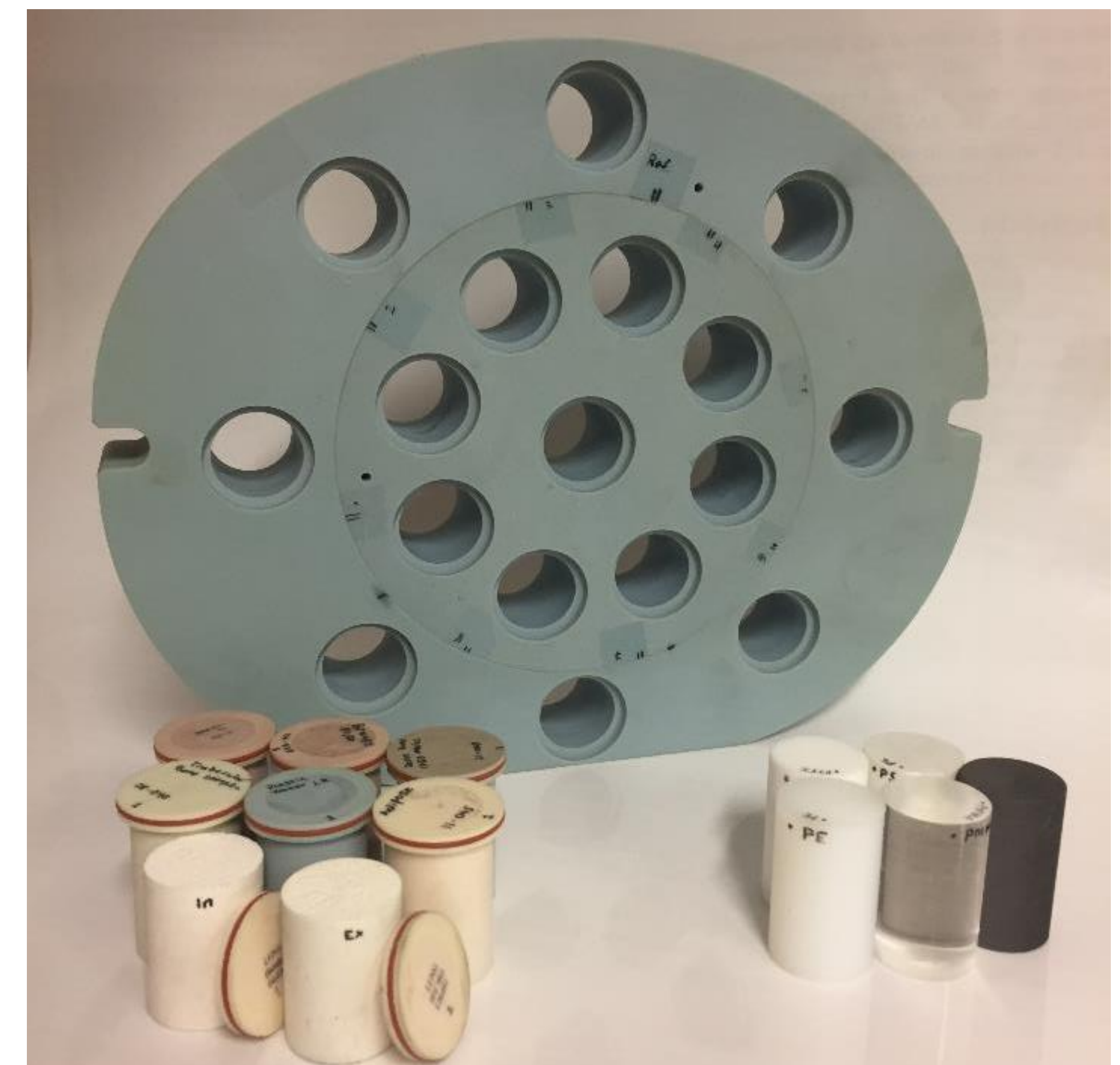
Figure 1. CIRS electron density phantom model 062A with eight tissue surrogate inserts. The top of the two lung tissue inserts was removed since they were made of other material. To the right five well-known materials made locally.
